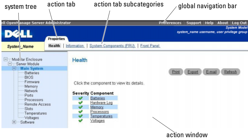
Figure 4-2. Sample Server Administrator Home Page — Modular System
